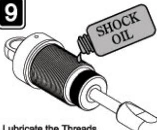
Lubricate the Threads with a SMALL amount of shock oil
