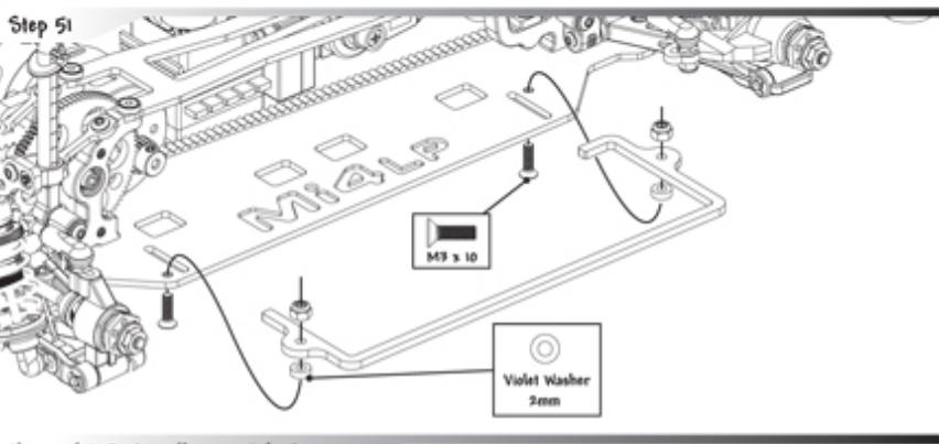
Humped LiPo Installation With Tape
