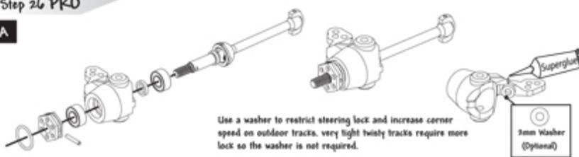
Use a washer to restrict steering lock and increase corner speed on outdoor tracks. very tight twisty tracks require more lock so the washer is not required.
