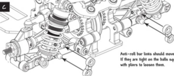
Anti-roll bar links should move freely.
